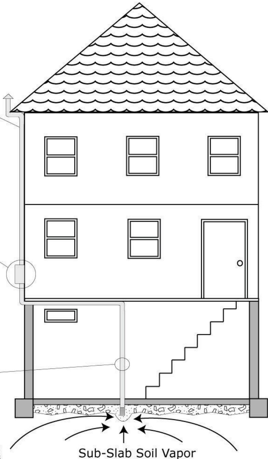
A sub-slab depressurization system vents contaminated soil vapor before it enters a structure. The fan draws vapor from beneath the building outside to the roof line where it is released to the outside air.
