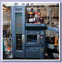
The samples are then analyzed by liquid chromatography - mass spectrometry. Basically, this separates, detects and identifies how much of a chemical is there.
