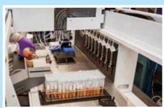
A portion of the serum is then transferred from the vial to a tray that contains 96 small wells. A special machine places one serum sample from each vial into each well. This machine tracks the ID # of the sample and its location in the tray along with several quality control samples.
