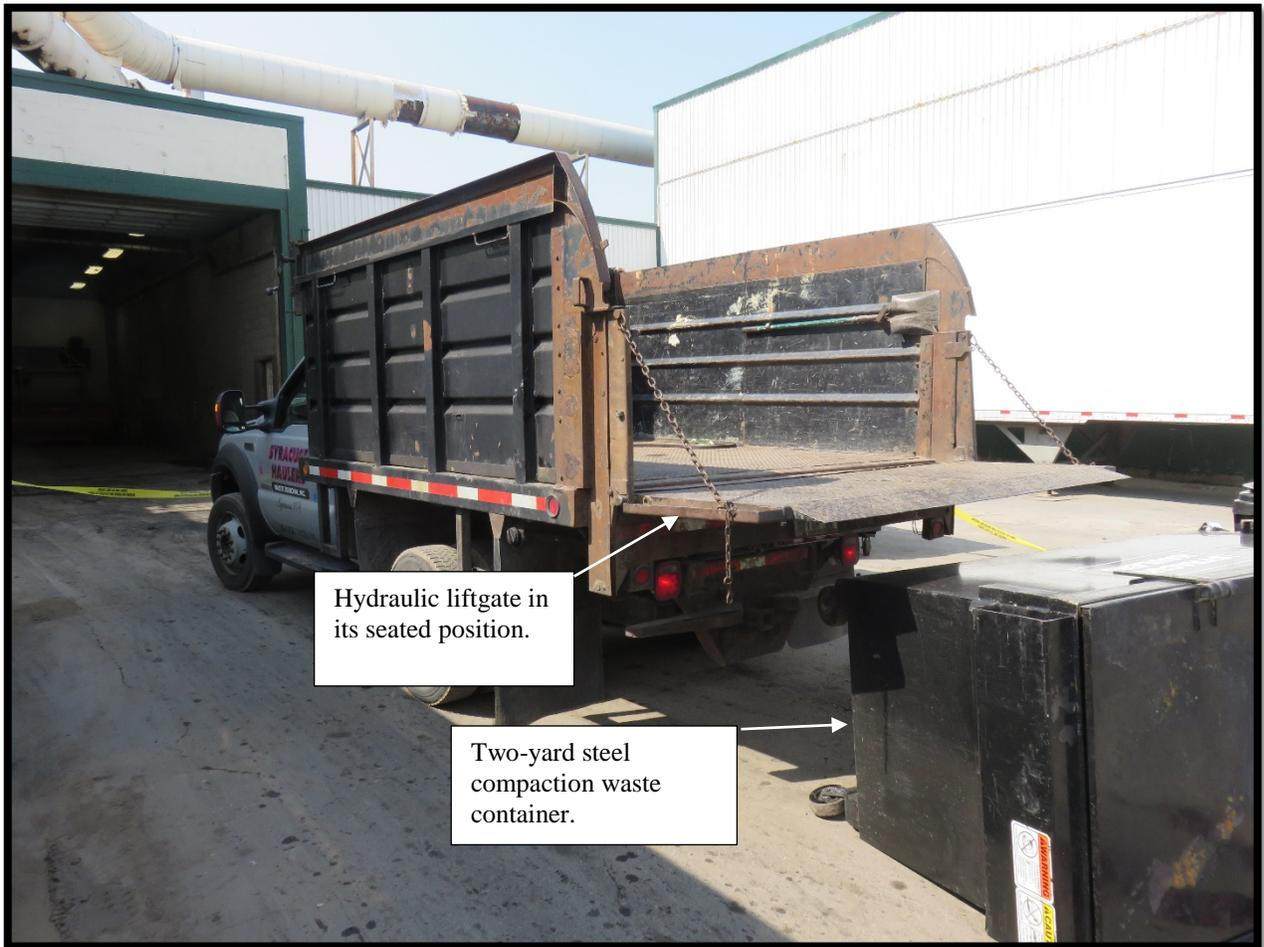
*Photo 1. The truck with hydraulic liftgate being used to load and unload containers and the container after falling from the liftgate. (Photo courtesy of OSHA)*
