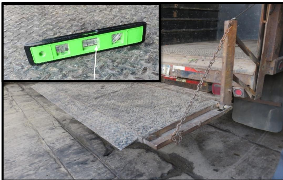
*Photo 2. The hydraulic liftgate in a lowered position. A level showing the downward pitch of the liftgate. The downward pitch was measured at an angle of 9.5 degrees. (Photo courtesy of OSHA)*
