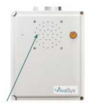
Never spray cleaner directly onto the AvaSure AMU as this could damage the electronics in the top assembly or in the body box. Never spray cleaner into the speaker grill at the front of the AvaSure AMU. Avoid excessive moisture/dripping cleaner to prevent ingress into sensitive electronic areas.
