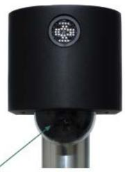
The camera dome should only be cleaned with a clean soft microfiber cloth. Paper towels can contain fibers that will scratch or eventually dull the lens.
