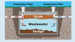
Have a DEC-permitted waste transporter inspect and pump out your septic system every 2-3 years to avoid potential well contamination from a failing septic system. Learn more at **Septic System Operation and** Maintenance
